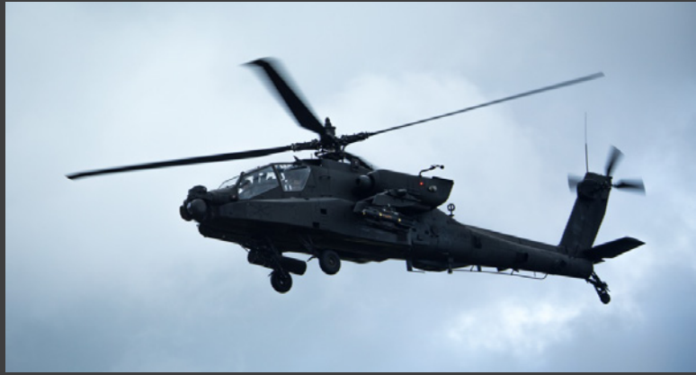
AH-64 Apache The AH-64 Apache is a twin-engine, four bladed, multi-mission attack helicopter assigned to JBLE-Eustis.
