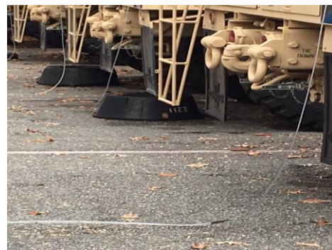
Photo 1035-6. Drip pans under vehicle not being used
