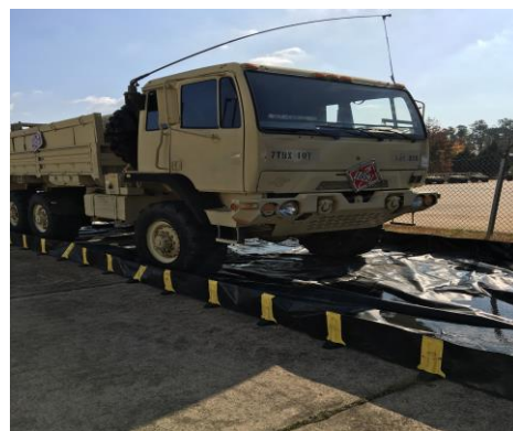
Photo 836-6. Collapsed secondary containment under mobile fuel tank
