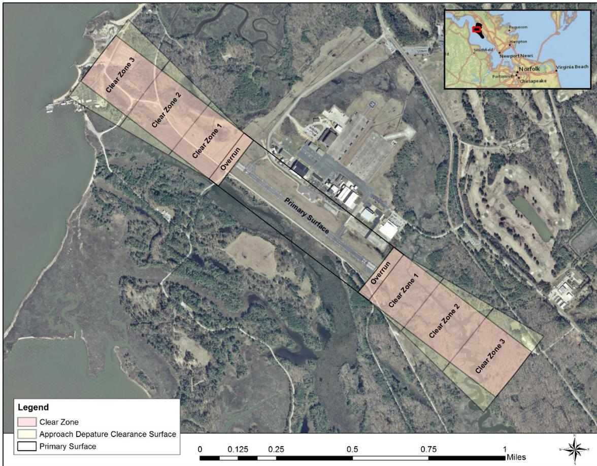
**Figure 3-1. Airfield Surfaces and the Clear Zone at the Felker Army Airfield**
