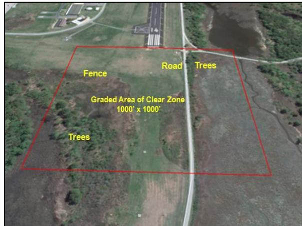
Figure 1. Runway 32 Graded Area Clear Zone      Figure 2. Runway 14 Graded Area Clear Zone
