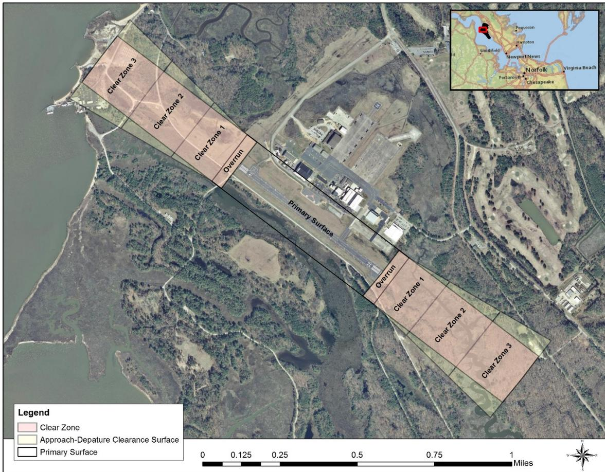
**Figure 2-2. Airfield Surfaces and the Clear Zone at the Felker Army Airfield**
